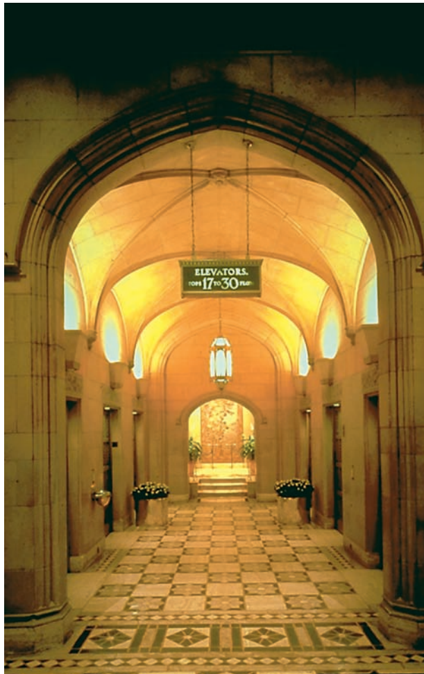
Plate 5-1 Elevator Lobby, Historic (Gothic-inspired). Chandelier in gothic style is decorative only. Ambient light and illumination of groin vaults by scone uplights. Task light created by downlight over elevator doors. Focal light on wall at end of hall provided by wallwashing. Photo: J. Benya
